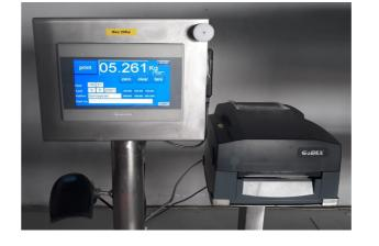
Tamay Efficient Processing Machine has its own label printer for use in the quality control table which is at the end of the machine. Label printer has barcode or RFID functions. This feature is optional.
