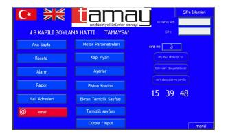
The HMI screen of the machine has all the necessary functions for the users. Since the setting pages contain important settings of the machine, it ask a password from the user. In this way, your machine's settings are preserved.
