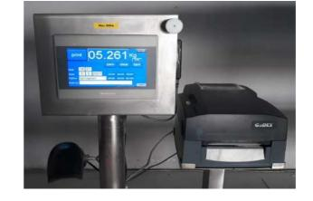
Tamay Precision Packaging Machine has its own label printer for use in the matching station at the end of the grader line. Label printer has barcode or RFID functions. This feature is optional.
