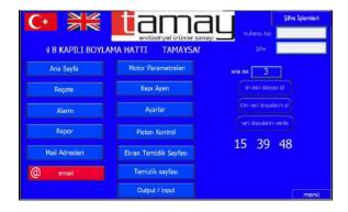
The HMI screen of the grading machine has all the necessary functions for the users. Since the setting pages contain important settings of the machine, it ask a password from the user. In this way, your machine's settings are preserved.
